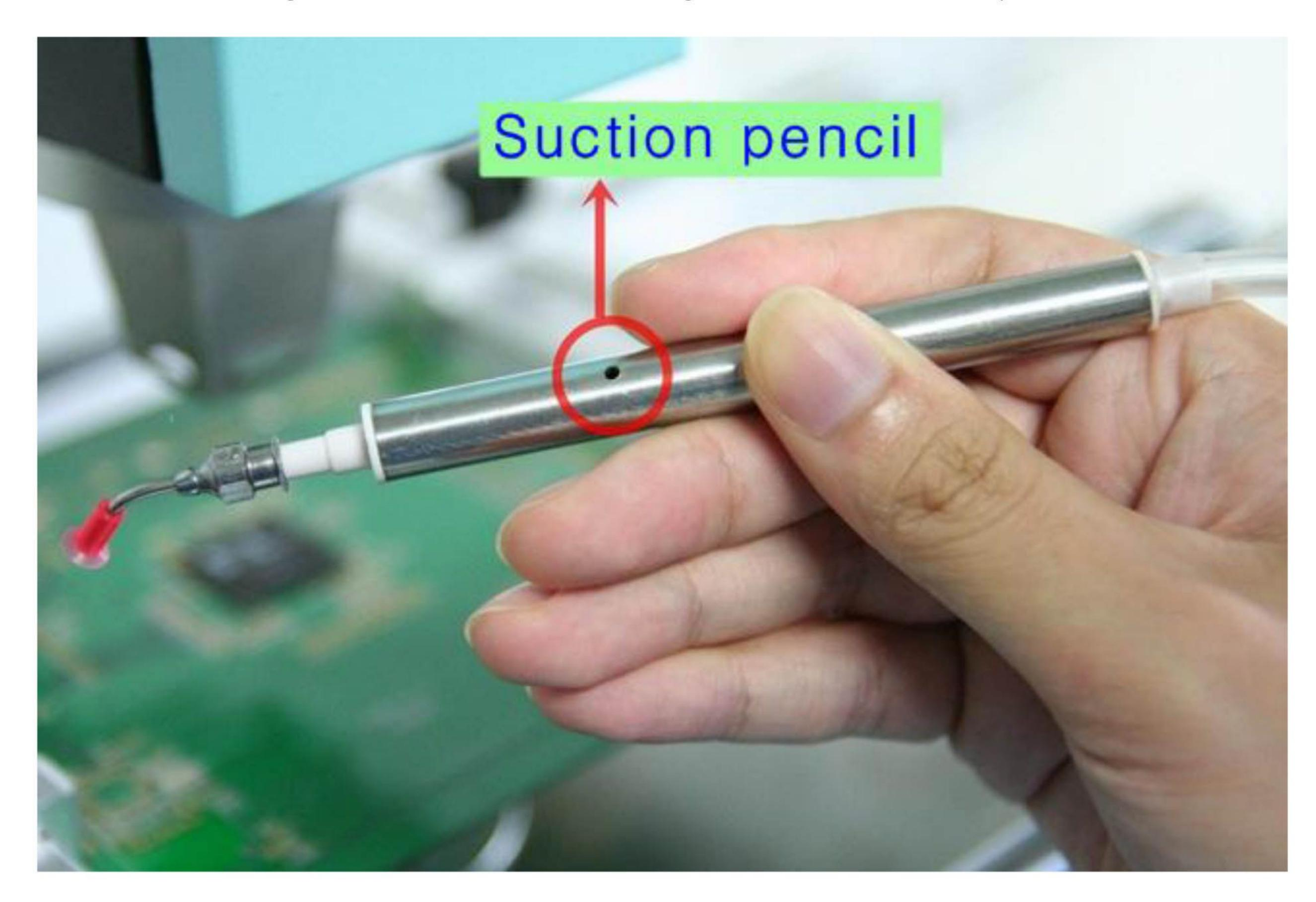
2.4 Raise the upper heater after buzzer sound and remove the target components using suction nozzle as soon as possible. Cooling fan is operated automatically after 10seconds, and suction function is also automatically stopped after 3minutes and 30seconds without particular manual operation.
