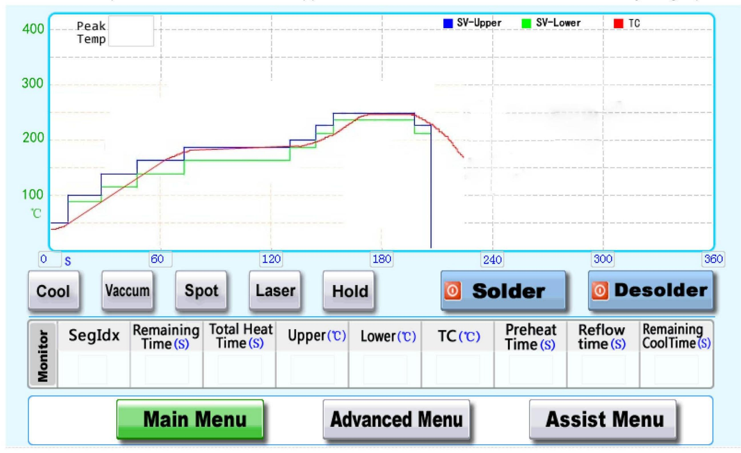
2.3 The heating is started by pushing the 'removing components' buttons. The buzzer sounds three times 13seconds, and suction nozzle is operated 10seconds automatically before completion. Then stan by holding upper heater moving knob after blocking the air hole until right before the completion.
