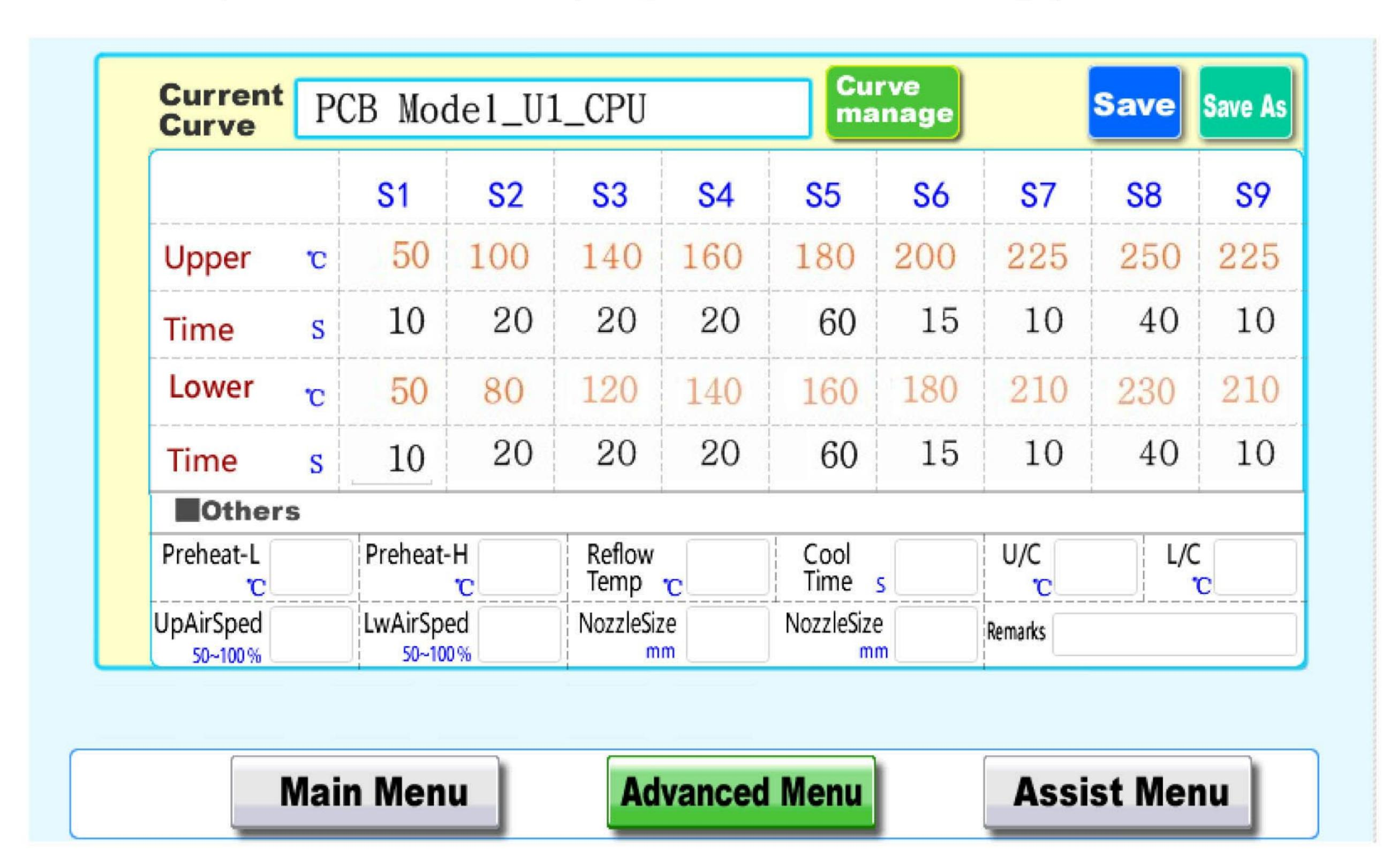
2.2 The setting value is applied automatically on the screen after importing the program and screen changing to working display, and also the value of temperature and time of upper and lower heater can be checked by a graph.
